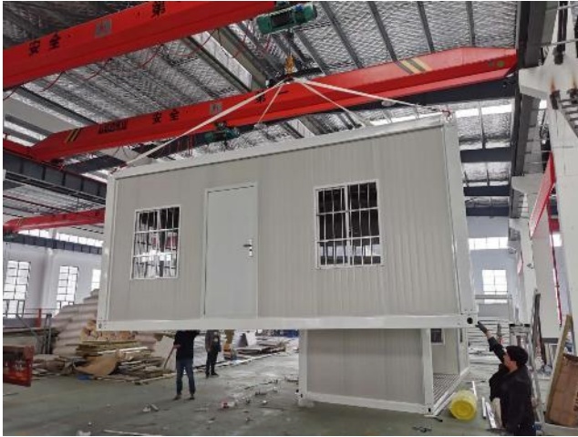
PBV System using light weight insulated wall panels can be designed as a 2 storey buildings and be fitted with En-suite prefab toilet module. The module can be lifted as one complete unit for relocation purposes
